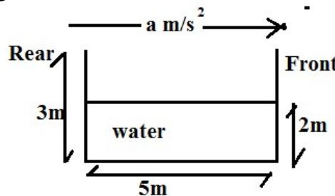
Maximum acceleration a that can be given without spilling the water is:
